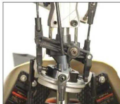
This is an over-exaggerated photo of what happens when collective input is given on an eCCPM setup when servo-grouping is not implemented.
